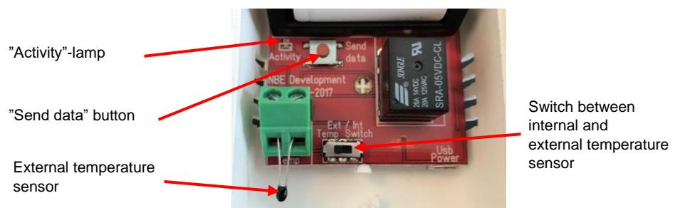
A) Remove the outer shield from the room temperature sensor and insert the batteries. Now check that the 'activity' lamp is flashing. See picture above. The room temperature sensor is equipped with an external and internal sensor. Always make sure that the room temperature sensor is set to use the internal sensor. This you can choose at the bottom of the print, where you can switch between "Ext / Int". The button must be on "Int".
